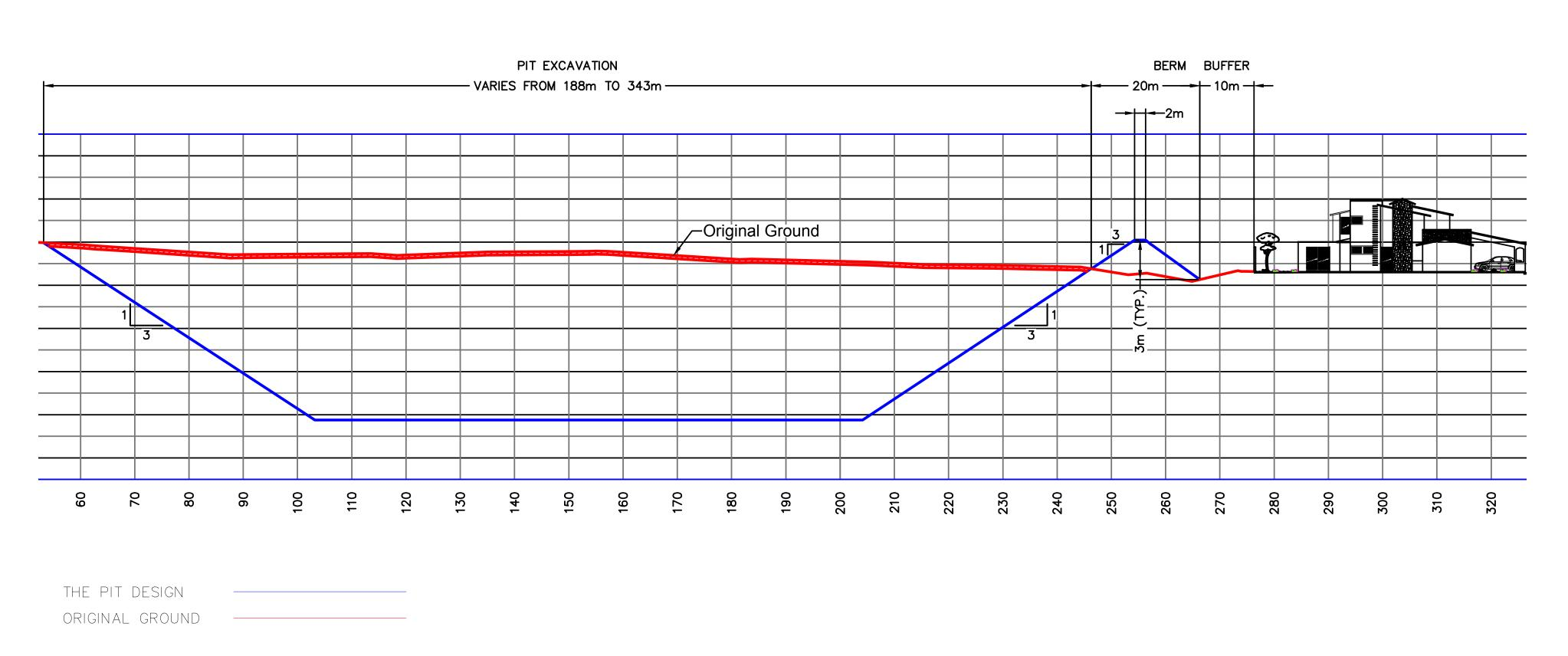
Example of a cross section of the gravel pit, including berm
